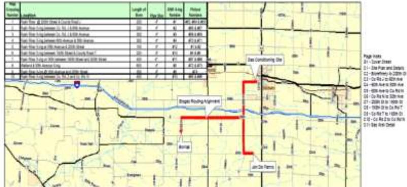
The above map shows the Biogas Pipeline route from Jon-De and Bomaz Dairies to the Gas Conditioning Site.
